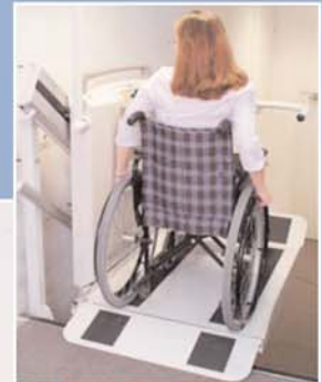
Call platform. Barrier arm rises (when controlled by the attendant or the joystick user) while front barrier arm and ramp remain in safety position.
