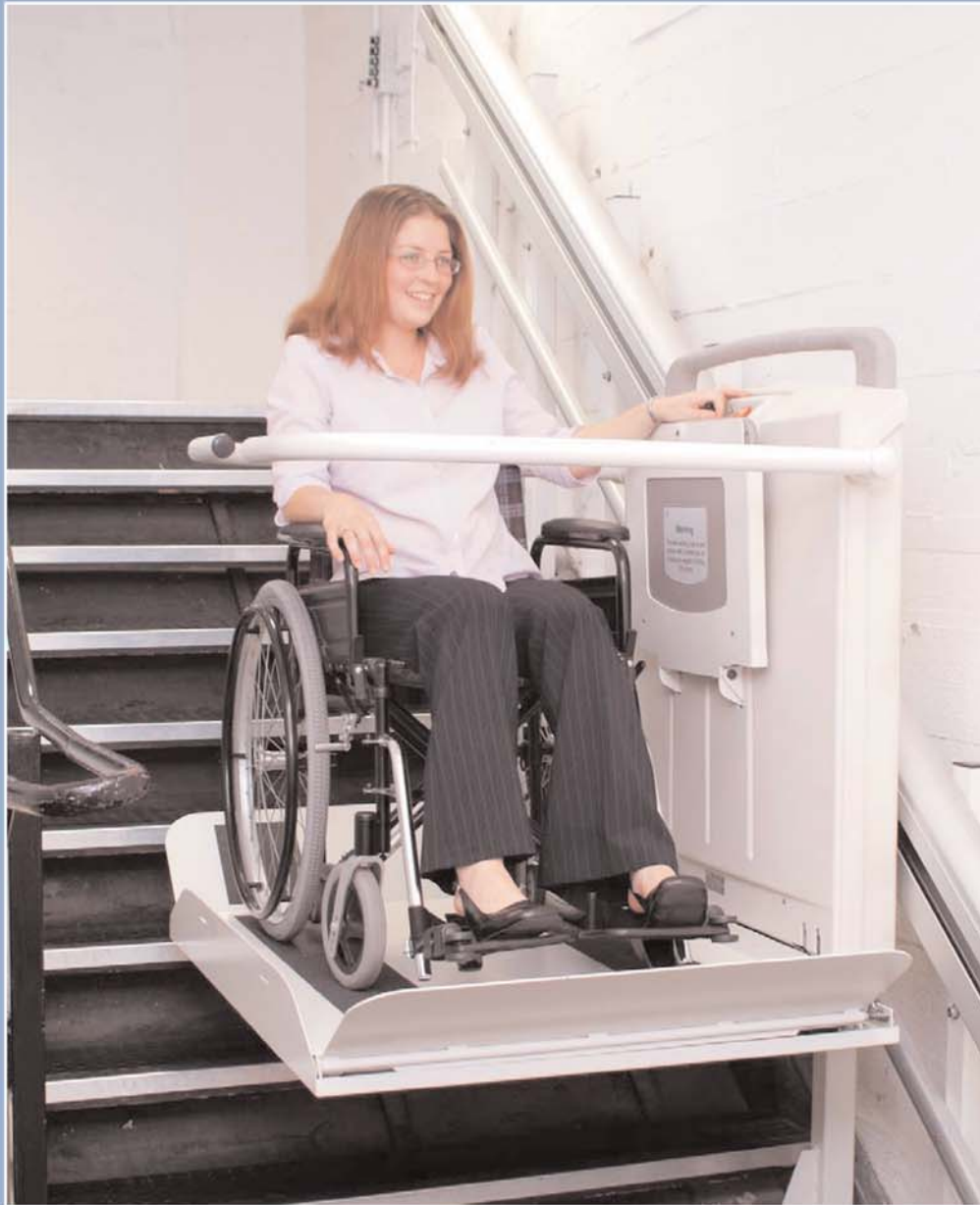
Call platform. Barrier arm rises (when controlled by the attendant or the joystick user) while front barrier arm and ramp remain in safety position.
